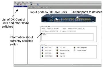
Figure 25 DX System Configuration window
